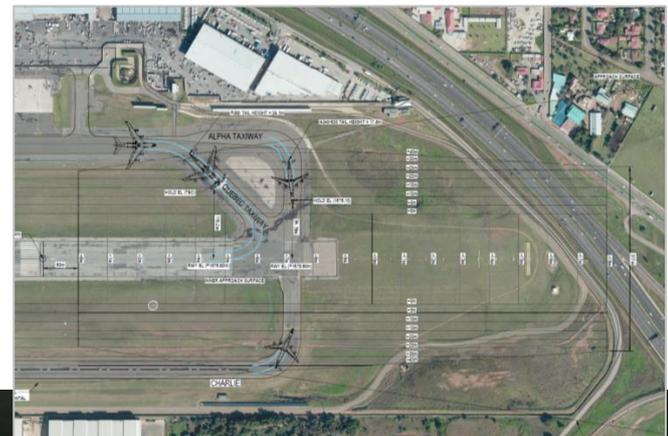
Aircraft tracking software was employed to model turning movements at two of the five critical hold positions where wingtip clearance distances had to be checked for safety reasons, non-trafficable pavement areas had to be demarcated, or where a new taxiway centreline trace was requested by the client.
